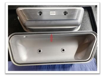
5. Attach the valve cover to the cylinder head (ensure you checked the valve clearance) if you use JPS Aircooled Cylinder heads this is super easy and fits like a clove! If you use stock cylinder heads a little trimming may be necessary because of the casting marks or any other drama that have happened in the past .... After this trimming, the valve cover will slide on with a tight fit.
