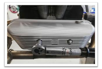
7. Finally, you can add the option you have chosen (breather or plug) or you make your own solution the thread is M18 x 1,5mm. Warning: never start or drive the engine with open breather or without plug.
