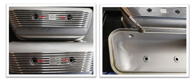
4. Take the black O-ring and put it in the O-ring groove (the length of the O-ring is already set) make sure that the ends come together with no gap. (Start point and endpoint at the red arrow position)
