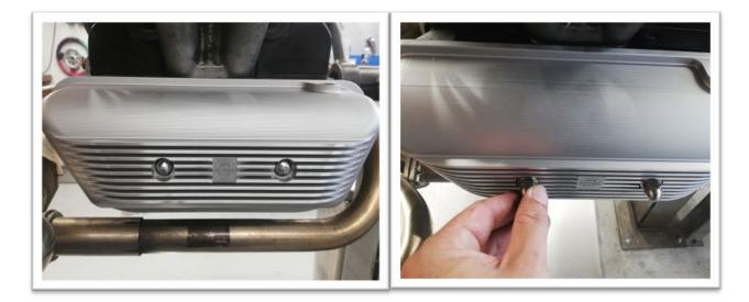
6. Torque the M8 cap nut with 14 Nm (10 ft-lb)
