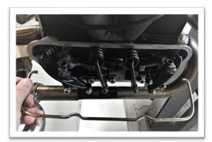
2. Remove the 2 outer M8 nuts for the intake rocker shaft. Remove the left M8 and replace it with the M8 stud extension, and torque it to 25Nm (18 ft-lb) according to the Porsche Workshop Manual.
